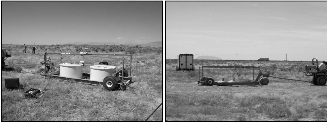
Figure 3.23. The RTDGPR antennas and cart (left), and the actual survey site (right) where the brush has been removed.
