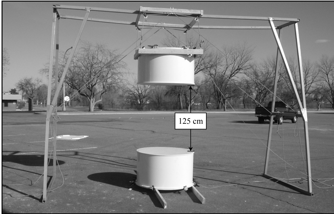
Figure 2.17. Face to face antenna reference arrangement used to estimate the impulse generator waveform. The frame is made from fiberglass.
